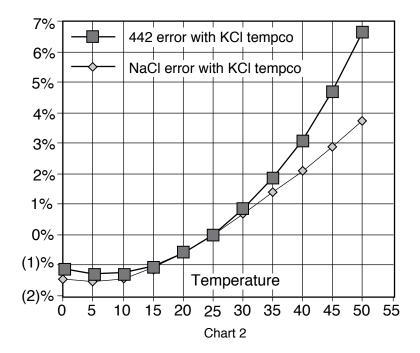
Users wanting to measure natural water based solutions to 1% would have to alter the internal compensation to the more suitable preloaded "442" values or stay close to 25°C. Users who have standardized to KCI-based compensation may want to stick with it, regardless of increasing error as you get further from 25°C. The PoolPro will provide the repeatability and convertibility of data necessary for relative values for process control.
